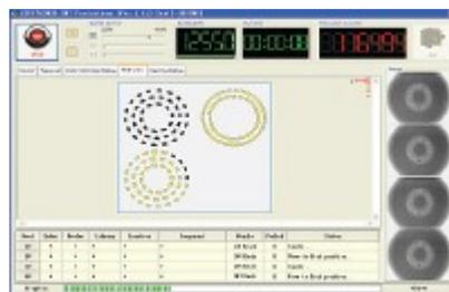
Real time monitoring screen for previewing production progress, production speed and production quantity during production
