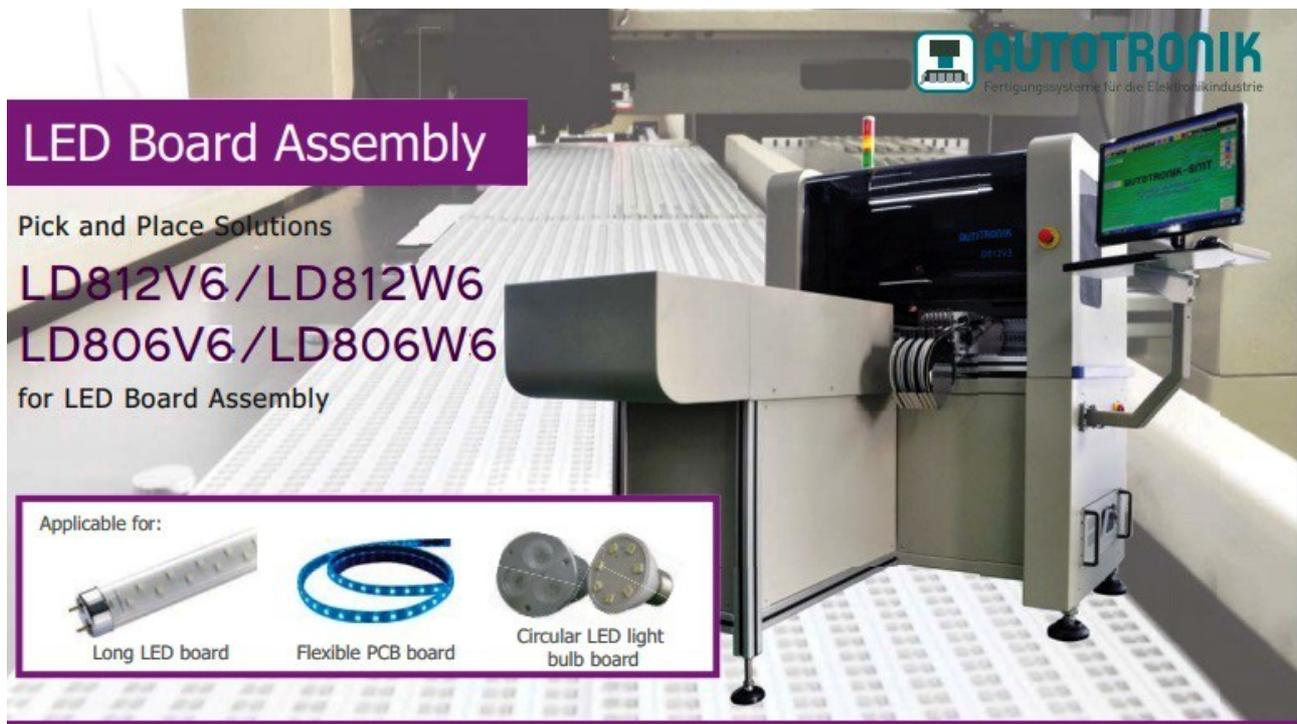
The SMD placement machine LD812 has been specially designed for use in the LED PCBs medium and high production quantities . The machine supports the processing of printed circuit boards with a length of up to 1200 mm (optionally up to 1800 mm ) .
